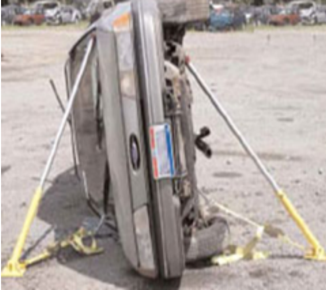
Note the rounded surface of the car body, install the strut on this side first when possible.
