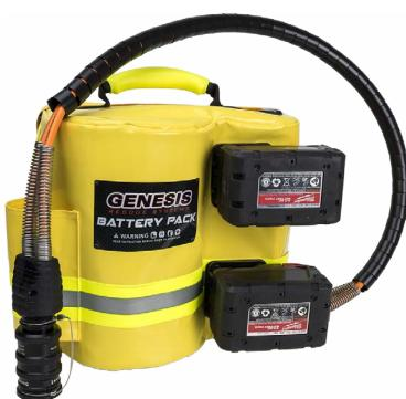
This power unit effectively transforms an existing conventional rescue tool into a battery powered work horse. The pack has the option to run on either 2 Milwaukee 28v batteries or just 1. Pump is also equip with power on demand. Always know the status of your fluid level with the bladder access window illuminated with LEDs.
